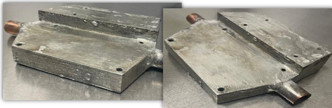
Figure 25 - Combined solution of internal sealant and external tin coating, showing acceptable results under 3.5 bar pressure.
