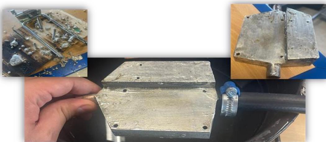
Figure 24 - Application of melted tin coating to the exterior surface of the liquid-cooled heatsink.
