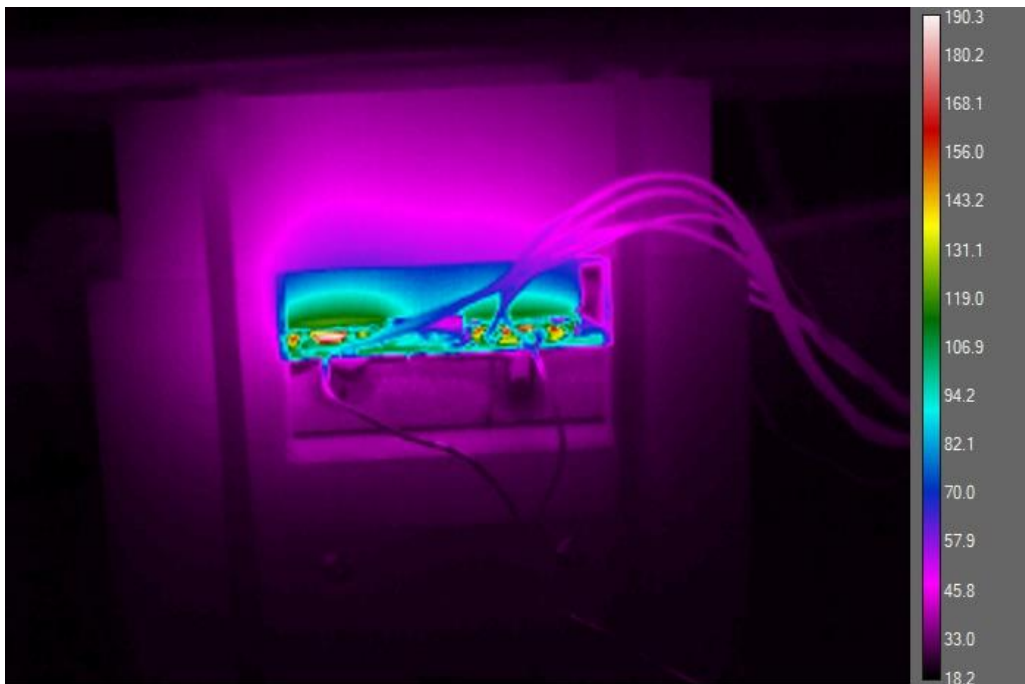
Figure 54 - Thermal imaging of heating elements on heatsink sample 2
