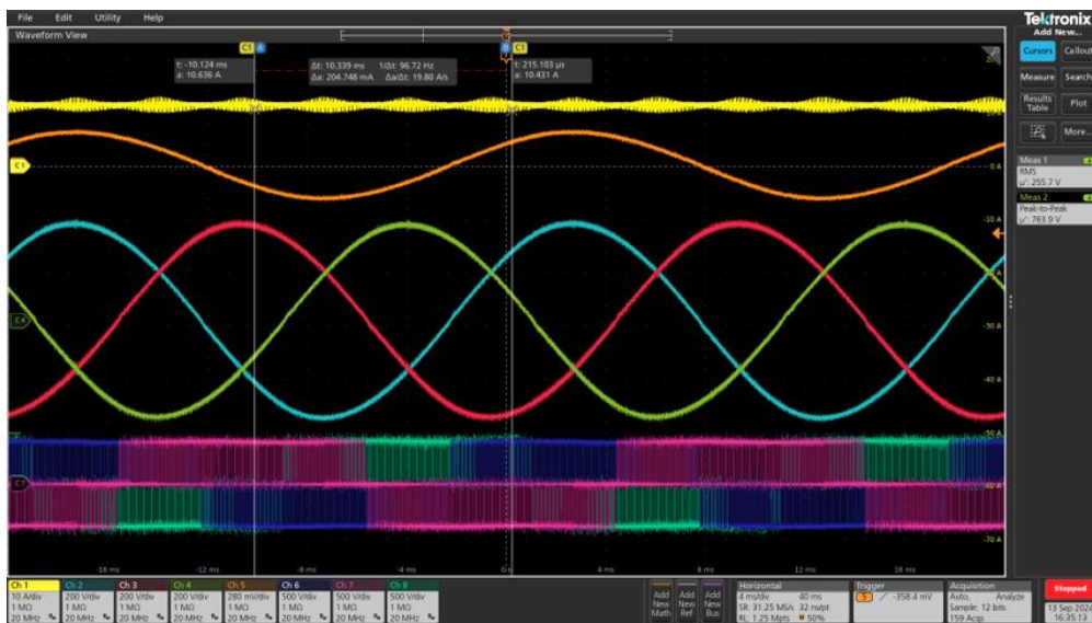
Figure 3.16 Low-power converter test waveforms at 10 kW resistive load
